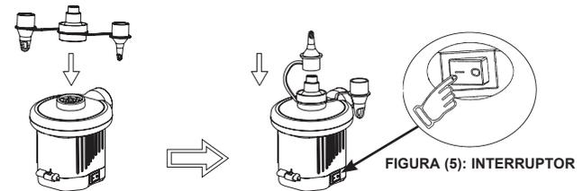
FIGURA (6): CONECTE LA BOQUILLA
