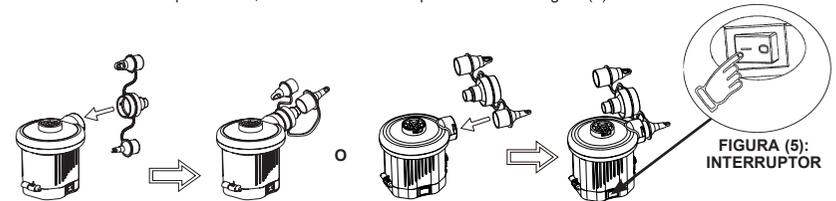
FIGURA (4): CONECTE LA BOQUILLA
