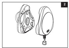
2. Place the transmitter (2) on the outside of the pool wall and the pool light (1) on the inside of the pool wall submerged in water. Ensure the transmitter magnetic poles are properly aligned with the magnetic poles on the pool light unit. See drawing (3).
