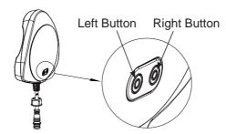
• Left button: turn the pool light ON and OFF, and sets the light mode.
