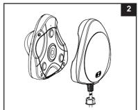
2. Place the transmitter (2) on the outside of the pool wall and the pool light (1) on the inside of the pool wall submerged in water. Ensure the transmitter magnetic poles are properly aligned with the magnetic poles on the pool light unit. See drawing (3).
