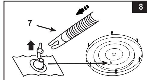
**NOTE:** If there is a need to add some air to the spa tub wall or spa cover air bladder after they have been setup, refer to above "Inflate the Spa Tub Wall" and "Inflate the Spa Cover Air Bladder" sections. The cover air bladder is preinstalled inside the spa cover. If it needs to be reinstalled, place the uninflated air bladder inside the spa cover lip before inflating the bladder.
